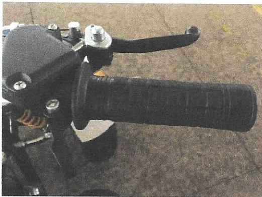
Brake trigger (upper), handle (middle), throttle lever (lower)
